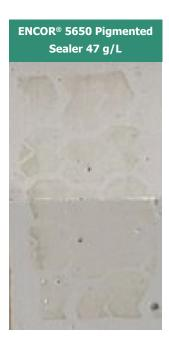
ENCOR® 5650 shows excellent imprint resistance and does not delaminate after wet compression of 150 PSI for one hour
